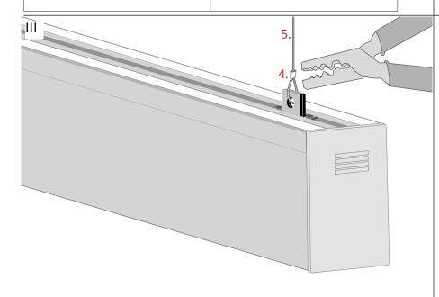
Run the cable (5) through the wire crimp (4) then through the hole in the fastener and again into the wire crimp. Use e.g. pliers to squeeze the wire crimp and close the created loop.
