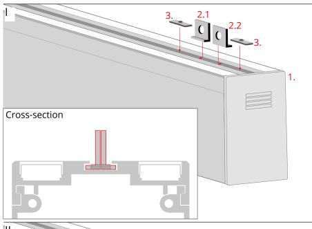
Insert the block (3), both UCHO-ZD fastener items (2.1, 2.2) followed by the second block (3) into the groove on the back of the fixture (1).
