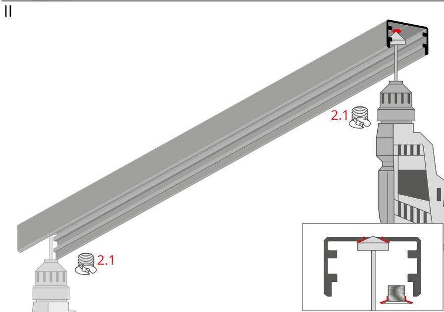
Chamfer the holes for threaded bolts (2.1).
