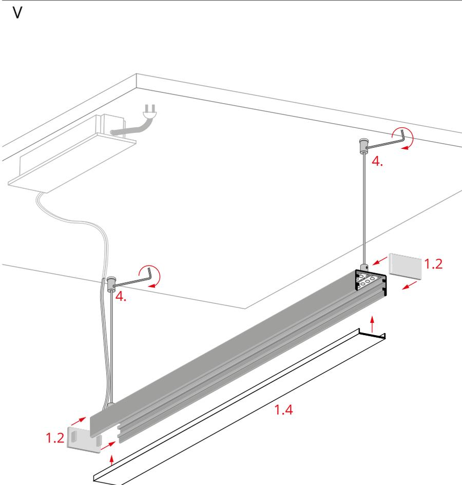
Mount the cover (1.4) and the end caps (1.2). Suspend the lighting fixture from the ceiling fasteners (4).
