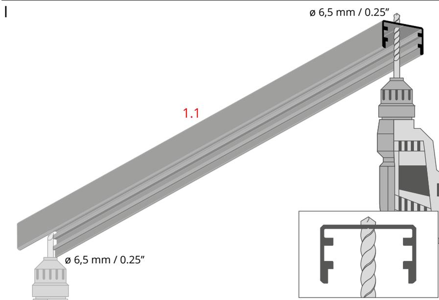
Drill holes in the profile (1.1) where the fasteners will be mounted.
