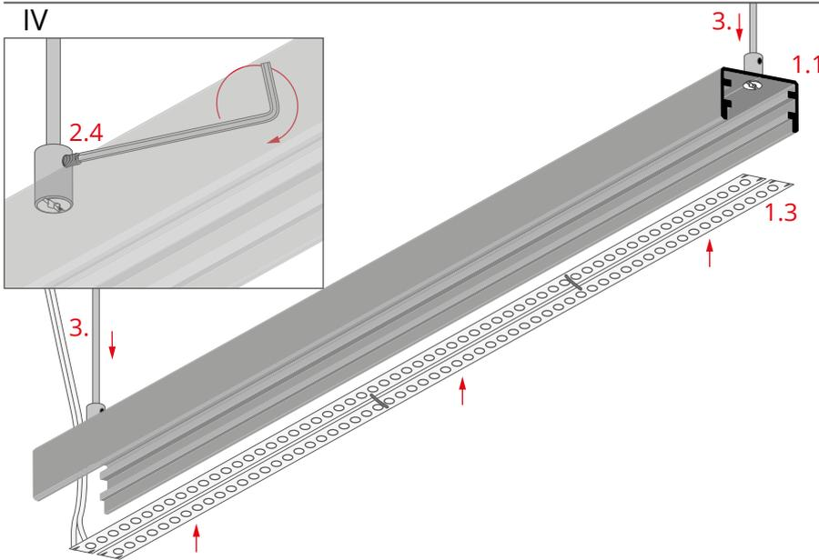
Mount and lock the rods (3), by tightening the pressure screws (2.4) in the heads of the fasteners.
