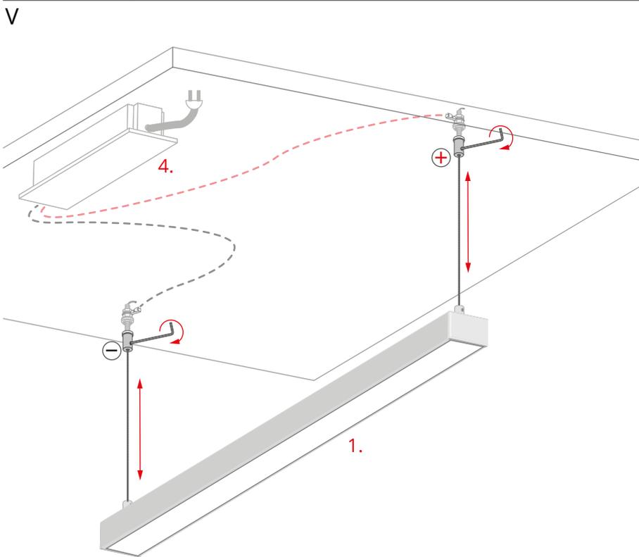
Suspend the fixture (1), adjust the length of the cables, so the fixture hangs evenly. Tighten the pressure screws (3.2) in the fastener bodies. Power supply cables must be connected to a 12 V / 24 V Power supply (4).
