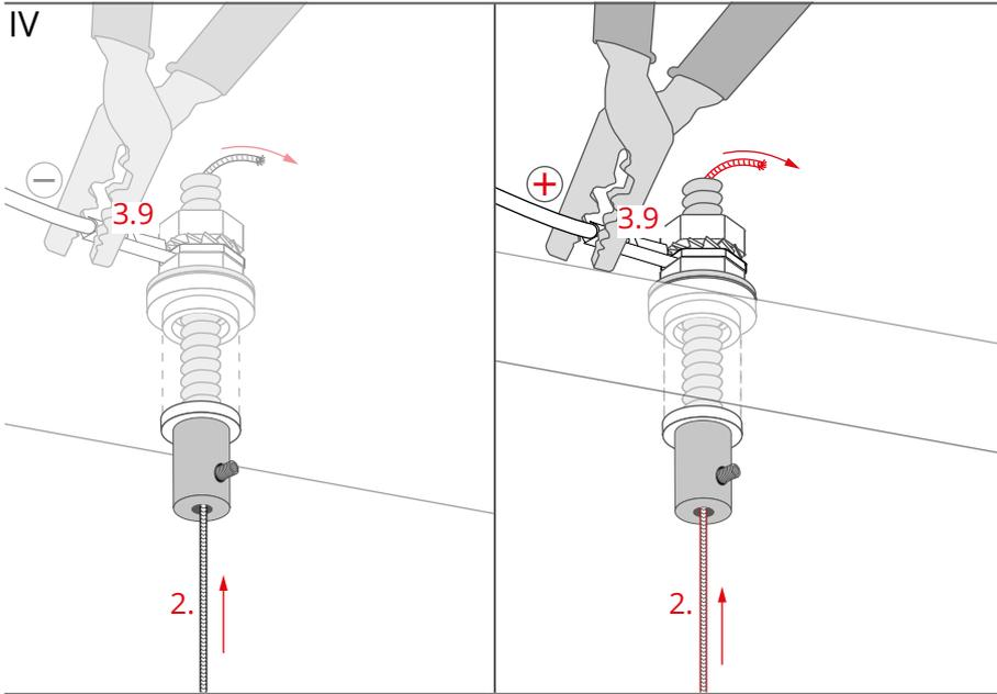
Lead the steel cables (2) through fastener bodies and threaded sleeves to the other side of the fastener.
