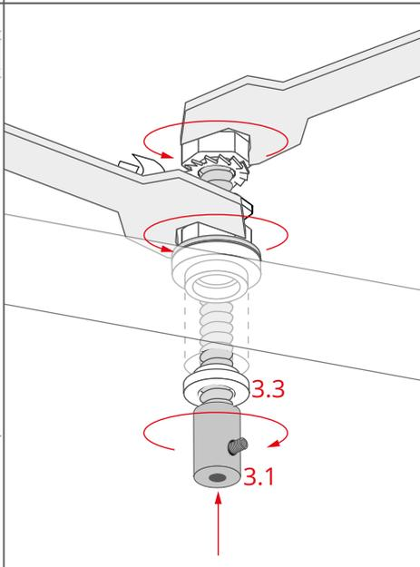
Put the pads (3.3) on the sleeves from the bottom and tighten them to the ceiling with fastener bodies (3.1).
