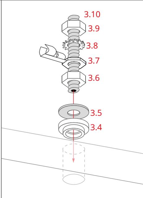
Put pads (3.4, 3.5) into the holes from the top and insert the threaded sleeves (3.10) with nuts (3.6), connectors (3.7), locking washers (3.8) and nuts (3.9) mounted.
