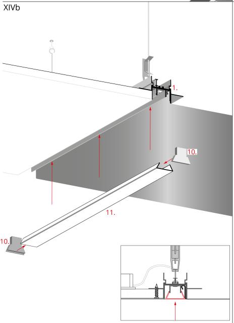
Mount the end caps (10) in the cover (11) and insert the cover into FOLED profile (1).
