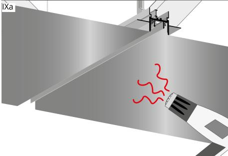
After proper installation of the stretched ceiling, stretch it with heater.
