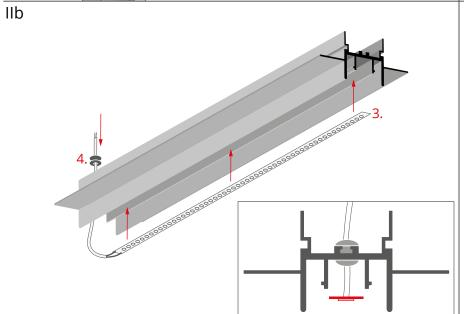
Mount the gland (4), adhere the LED tape (3) and lead the power cable through the gland.
