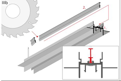
Shorten the FOLHAK profile (2) by minimum 20 mm / 0.79". Then mount it in the groove on the back of the FOLED profile (1).
