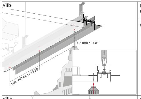
Drill holes through the board and the profile's flange.
