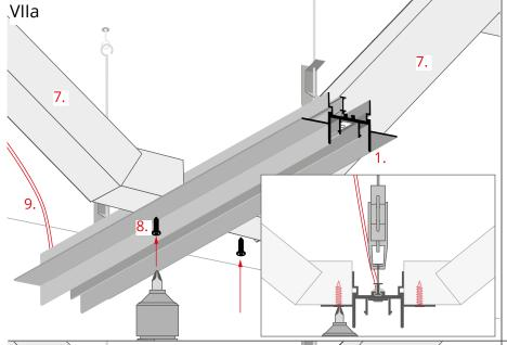
Screw the FOLED profile (1) to the structure of the suspended ceiling (7) with screws (8).
