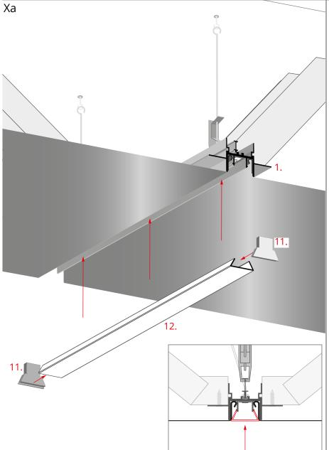
Mount the end caps (11) in the cover (12) and insert the cover into FOLED profile (1).
