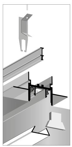
a) Suspension mounting with the stretched ceiling on both sides of the profile - p.  $\mathbf{2}$
