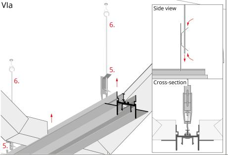
Suspend the fixture on the hanger rods ø 4 mm (6) with the spring hangers (5).
