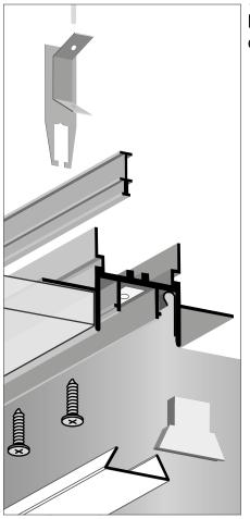
b) Mounting to drywall on one side with stretched ceiling on the other side - str. 7
