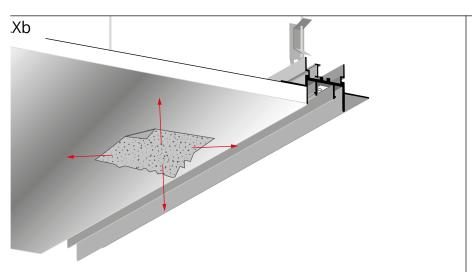
After the plaster has dried, sand the surface with sandpaper.
