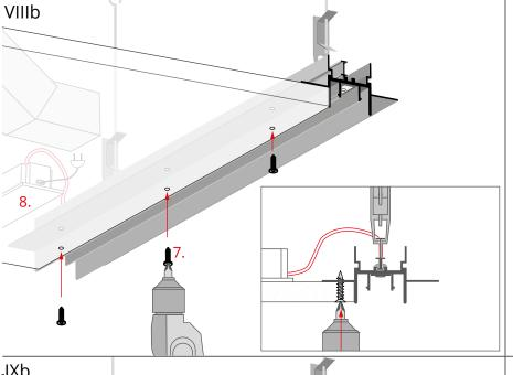
Insert the drywall screws (7) in the pre-drilled holes and screw the profile flange to the board.
