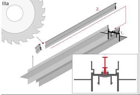
Stretch the ceiling foil with heater and mount the cover (2) in the profile.
