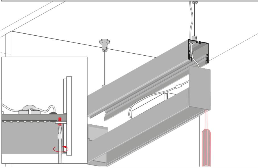
In case of „wall-to-wall” installation it is necessary to mount the fixture with the end caps from the bottom.
